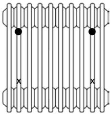
Wall Ties should be logically positioned to prevent Steel Multi Column from falling away from the wall, usually in line with Wall Brackets. If more than 2 brackets have been supplied these should be spaced evenly.
